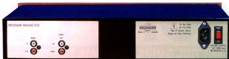
There's not a lot going on round the back of the RGCD5 ENR, however a notable inclusion is a coaxial digital input which accepts 16 or 20-bit data.
