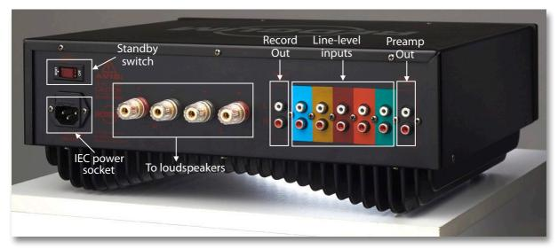
If you have a turntable ensure that the signal from its pickup cartridge is first connected to a phono pre-amp such as the REDGUM *RGPH2ENR*. The output of the phono pre-amp can be connected to any of the inputs on the back of your amplifier.
