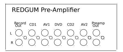
Connect the output jacks of each of your components to the corresponding input jacks at the rear of the amplifier. When doing this, be careful to ensure that the correct Left/Right channel connections have been made. RCA connectors are colour coded to help you, so use the white plugs for the Left channel and the red plug for the Right channel. We recommend the use of high quality RCA interconnects wherever possible, for the best quality sound. (e.g. REDGUM's **RGAP 05, RGAP 1 & RGSil**)
