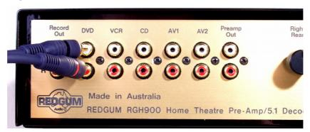
Connect the output jacks of each of your components to the corresponding input jacks at the rear of the amplifier. When doing this, be careful to ensure that the correct left/right channel connections have been made. RCA connectors are colour coded to help you, so use the white plugs for the left channel and the red plug for the right channel. We recommend the use of high quality RCA interconnects wherever possible, for the best quality sound. (e.g. REDGUM's **RGAP 05 & RGAP 1**)
