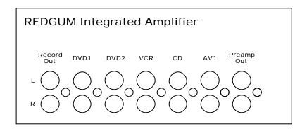
Connect the output jacks of each of your components to the corresponding input jacks at the rear of the amplifier. When doing this, be careful to ensure that the correct left/right channel connections have been made. RCA connectors are colour coded to help you, so use the white plugs for the left channel and the red plug for the right channel. We recommend the use of high quality RCA interconnects wherever possible, for the best quality sound.
